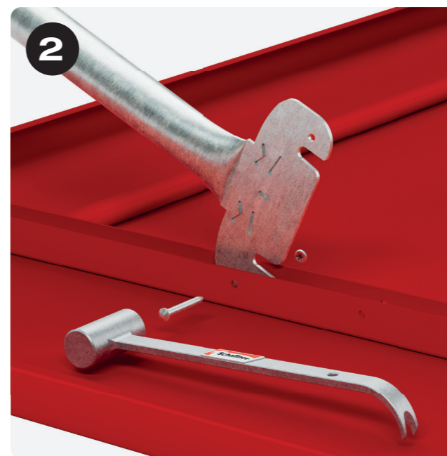
Place the pedestal on the table top so that the pedestal supports are between the struts. Then, secure in place on both sides with a notched nail and a notched nail holder.
